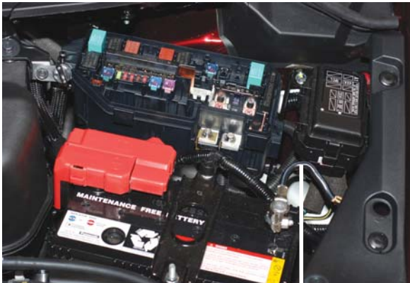
Negative 12-Volt Battery Cable
