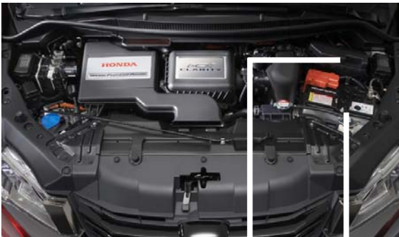
Underhood Fuse Box
