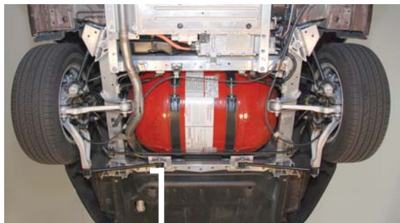
Hydrogen Pressure Relief Tube Location
