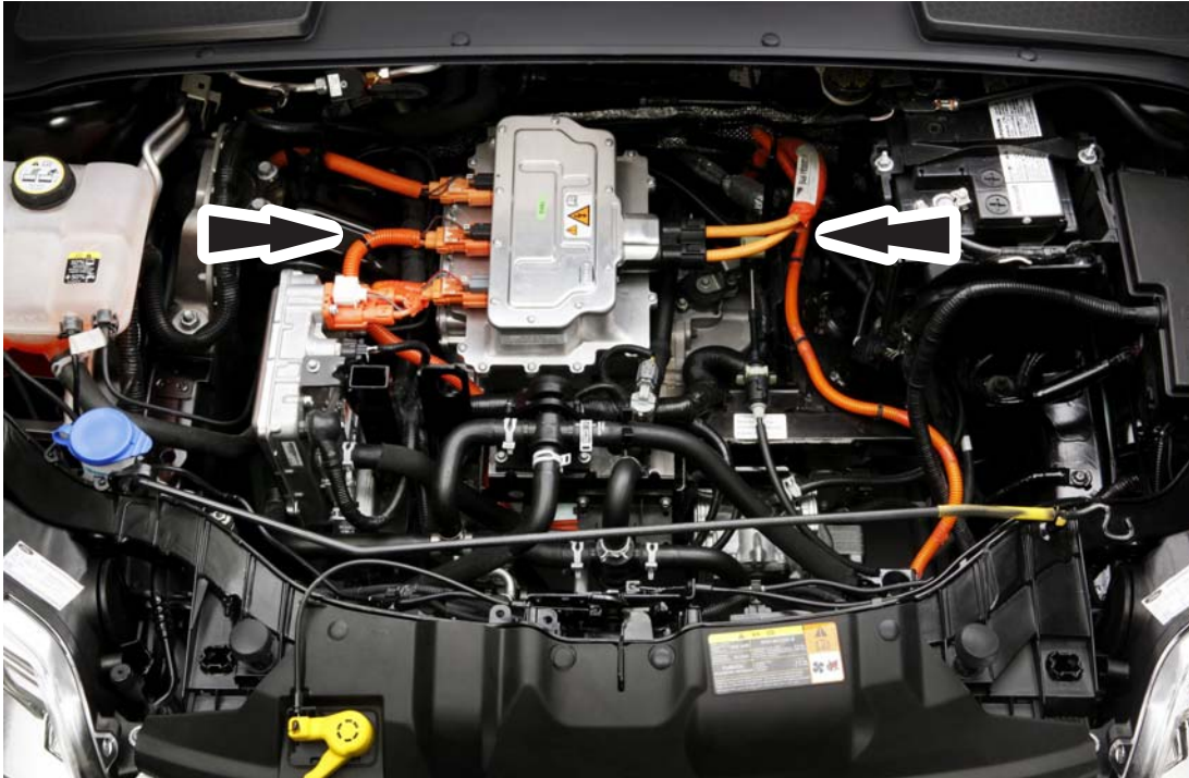
Orange high-voltage cabling from the high-voltage battery packs.
