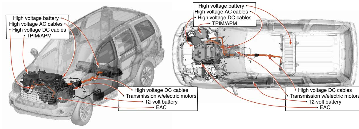
**– Safety Features –** In most accident situations an automatic shut-off of the high voltage system is triggered and the flow of energy from the high voltage system is disabled.
