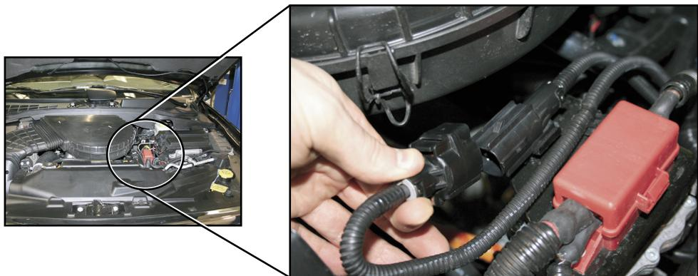
Disconnecting the 12-volt battery negative cable also disables the supplemental restraint system (SRS). The SRS may remain powered for up to two minutes after the vehicle is disabled.
